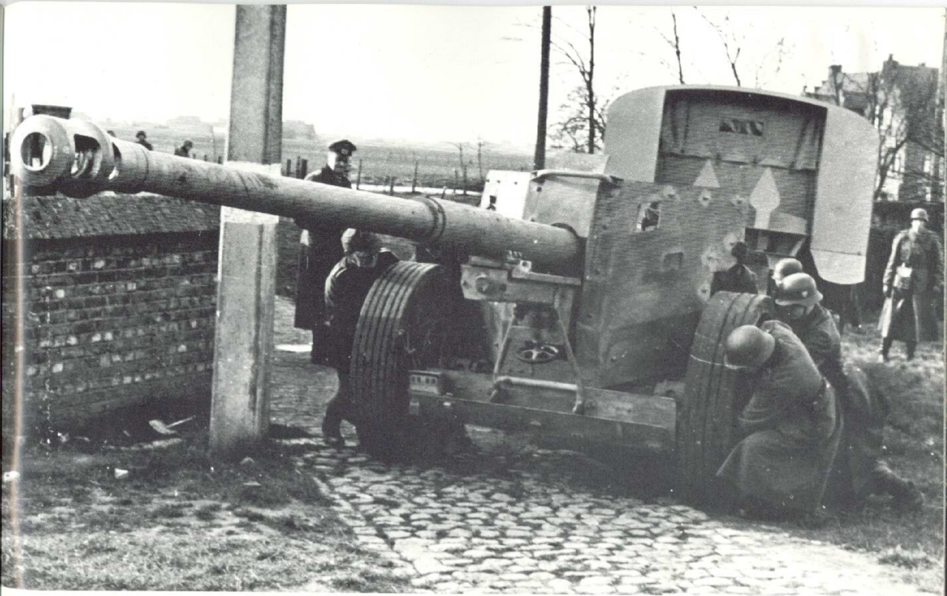
It was almost impossible for a crew to put a gun into position because of its great weight. The 88mm Pak was modified because of increasing shortages of materials. Instead of the earlier 88mm Pak 43, there were modified models 43/1, 43/2 and 43/3. The weight rose to 4380 kg and the height of the shield was two meters.
