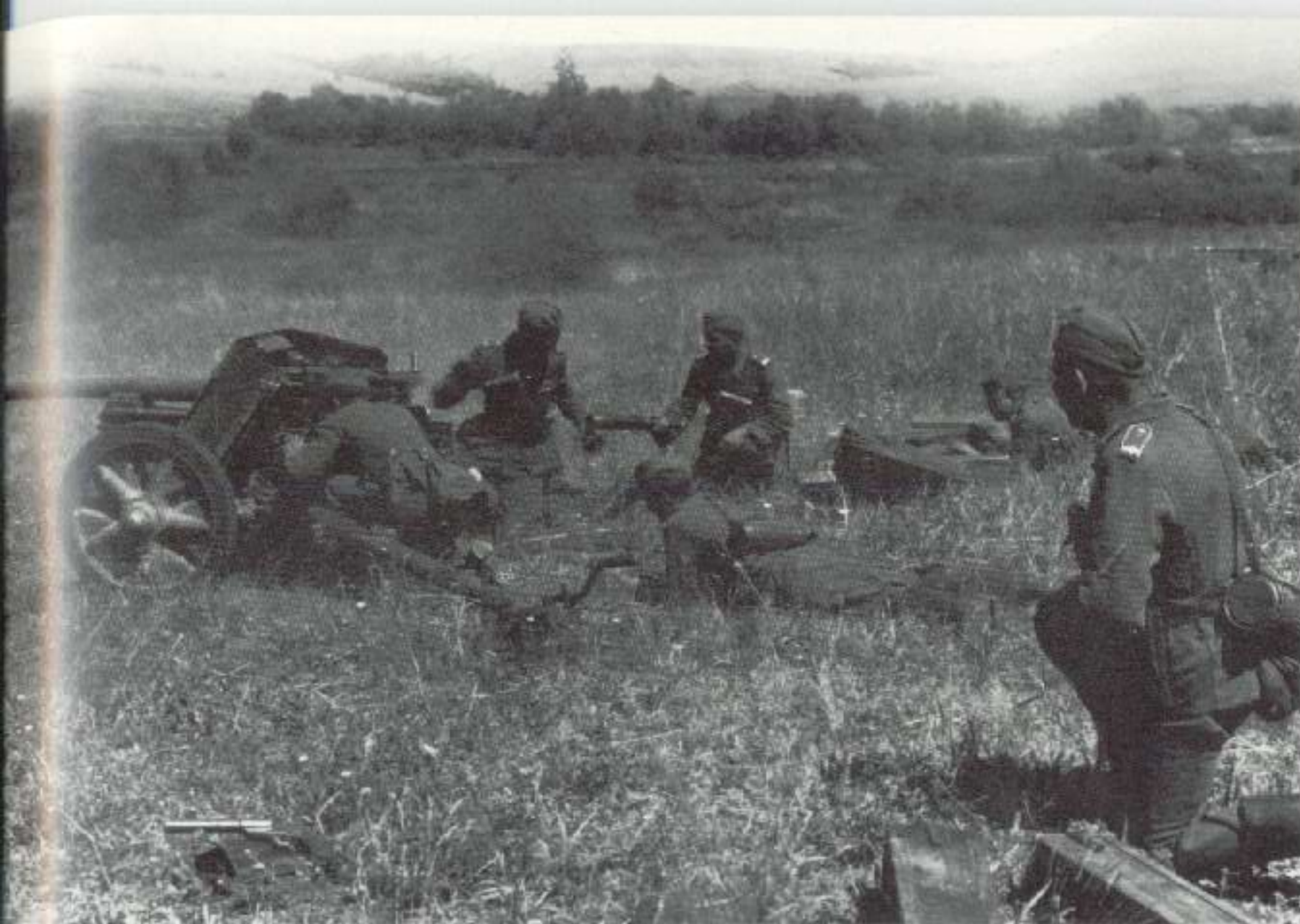
Above: Firing drill with the 50mm Pak at the Panzerjäger Training Unit's training facility. The features of the new Pak are clear to see: longer barrel, double shield, wheels, etc. The gunner is sighting the target, the loader takes the shell from the ammunition carrier, while the group leader, off to the left, observes his crew.
