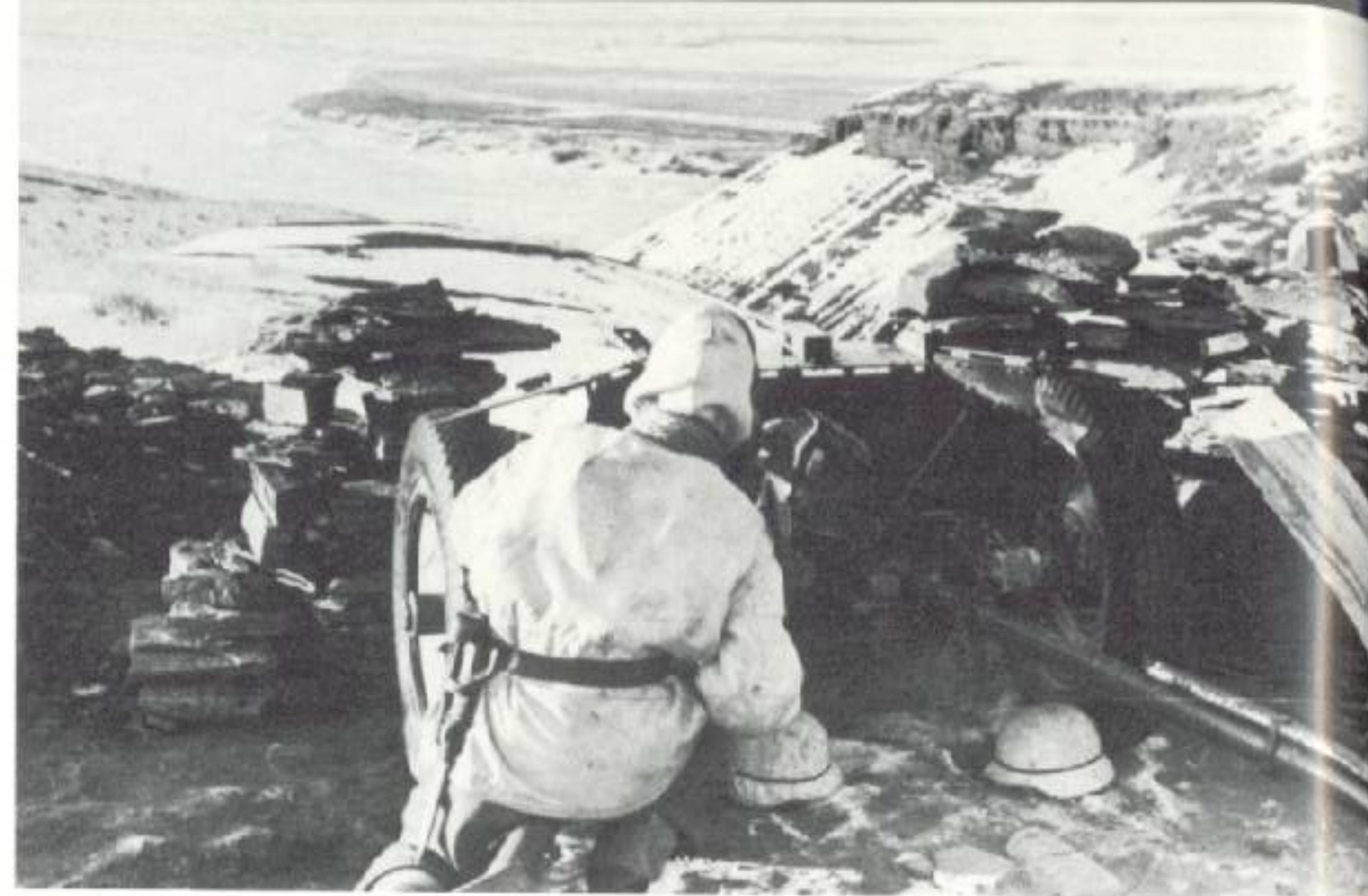
The low height, shortness of the spars and narrow spread of them allowed the gun to take up a small position. The upper part of the front shield could also be folded down—and the gun became even smaller. The guns are seen here on the steep bank of a big Russian river in 1943 (above) and before Tobruk, North Africa, in 1942 (below).
