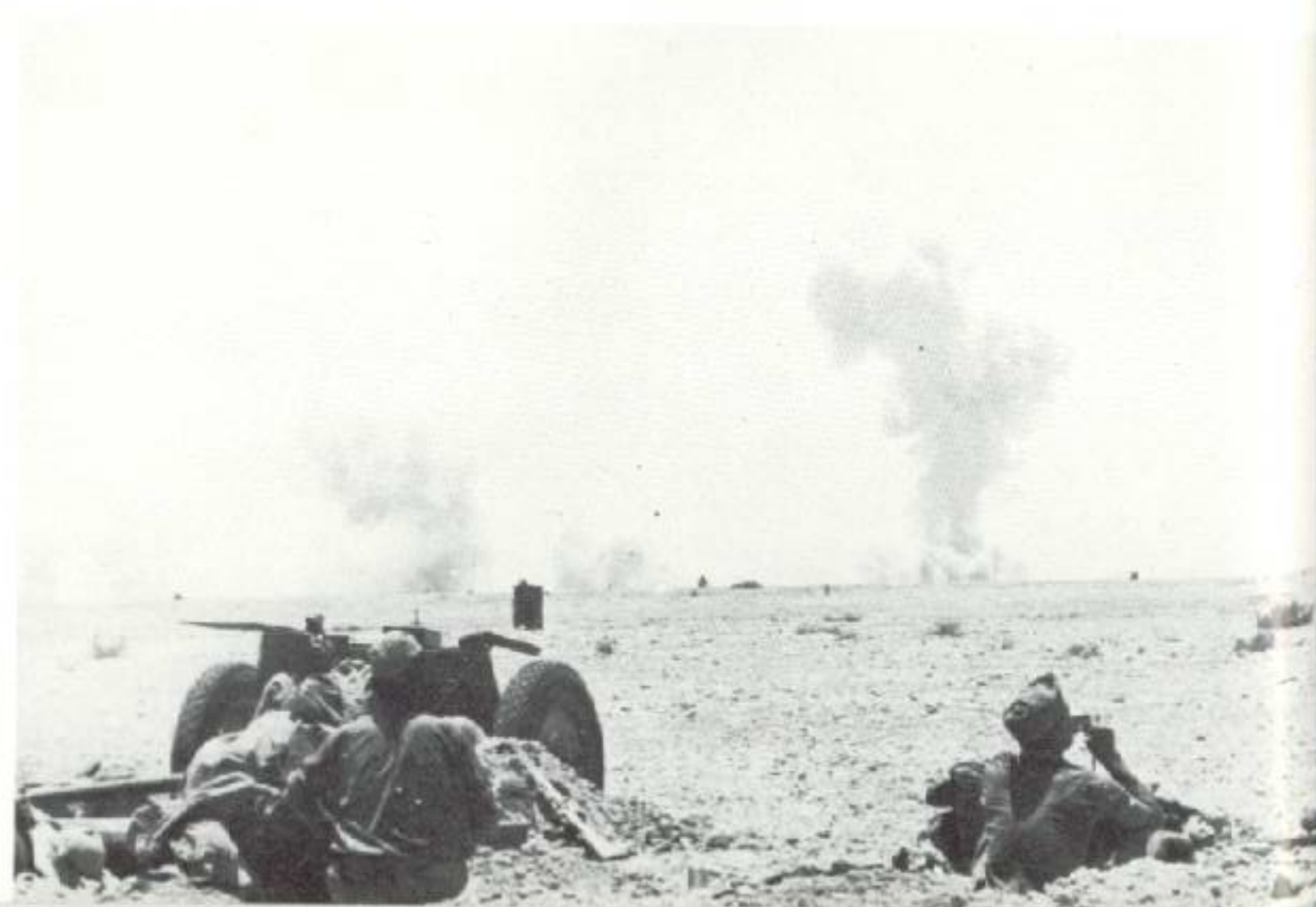
The low height, shortness of the spars and narrow spread of them allowed the gun to take up a small position. The upper part of the front shield could also be folded down—and the gun became even smaller. The guns are seen here on the steep bank of a big Russian river in 1943 (above) and before Tobruk, North Africa, in 1942 (below).
