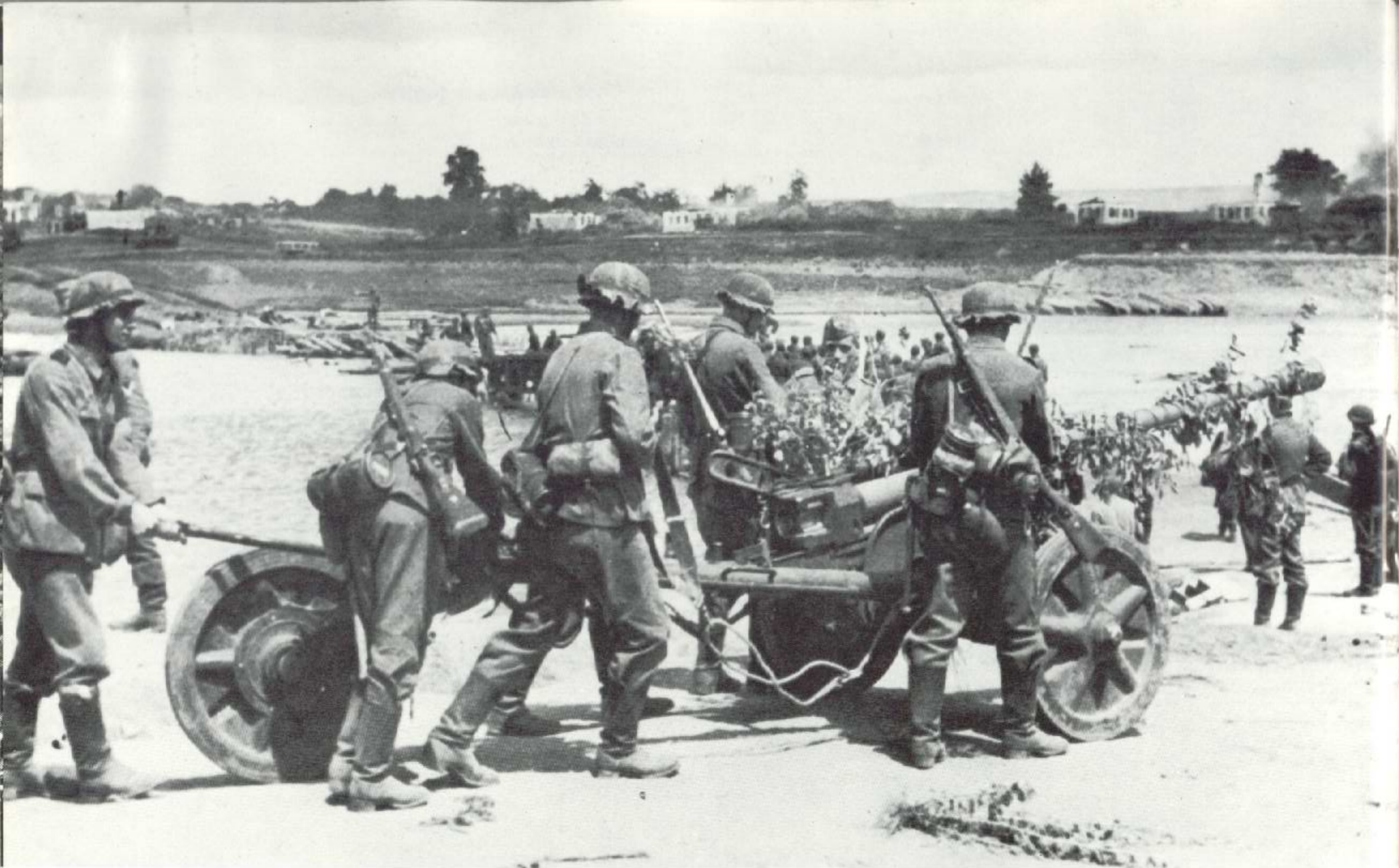
The 50mm Pak could be moved by its own crew on roads and firm ground. This is why the third wheel at the end of the spars was added (see above) and made so the gun could be steered. (Photo taken in the Ukraine, July 11, 1942).
