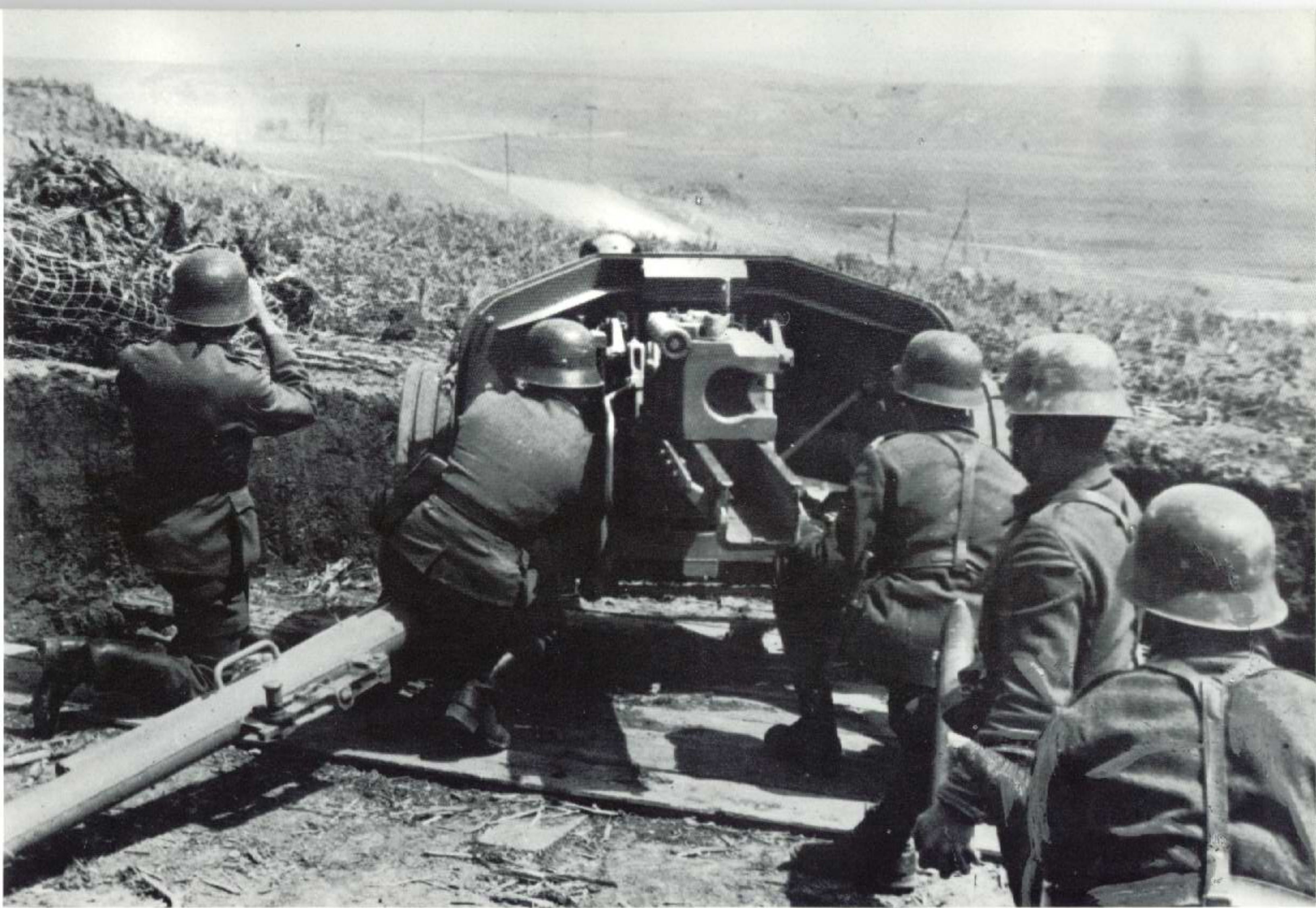
Emplacement of a 75mm Pak 40 in the Carpathian foothills (May 30, 1944). The breechblock, gun cradle, mount and shield are easy to see.
